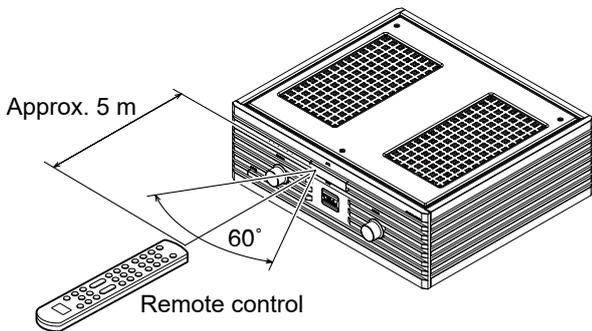
Operate the remote control within approx. 5 m distance from the front panel of the main unit within an angle of 60° to the remote sensor.
